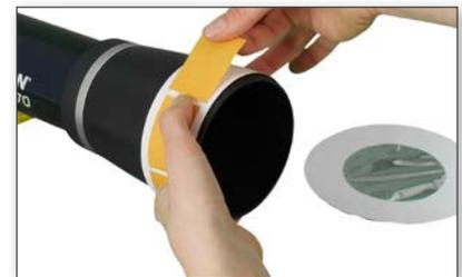
9. Finally, glue the AstroSolar Safety-Film holder onto the 50mm cylinder while the cylinder is still mounted onto the front end of your telescope.
